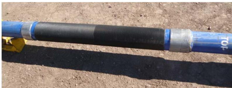
*Photograph of Steel External Casing Packer (Saltel Steel ECP) after pull out of hole preceding the 2nd run: No damage indicating the product has been run through tight spot*
