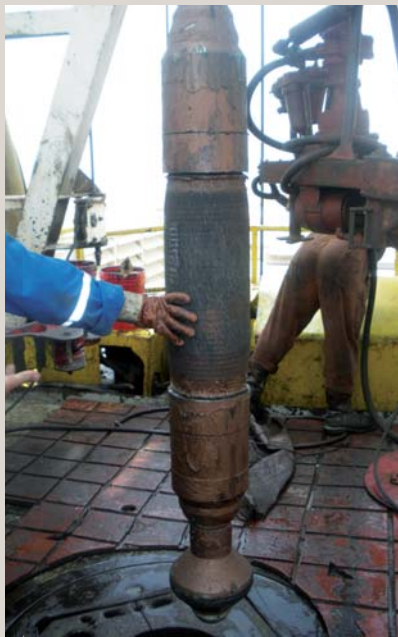
Downhole Expansion Tool and Packer after Setting.
